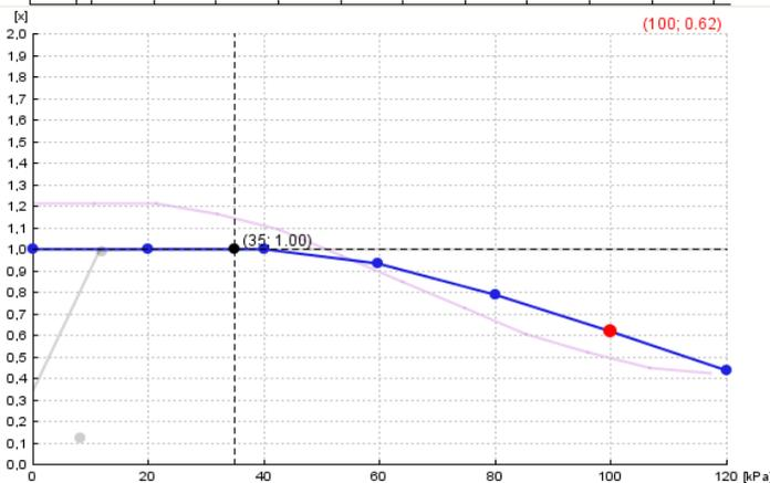
Multiplier Correction (eg. 1.0 is 100%, 0.6 is 60% of original shifting offset) of the angle regarding the engine manifold absolute pressure (load).
