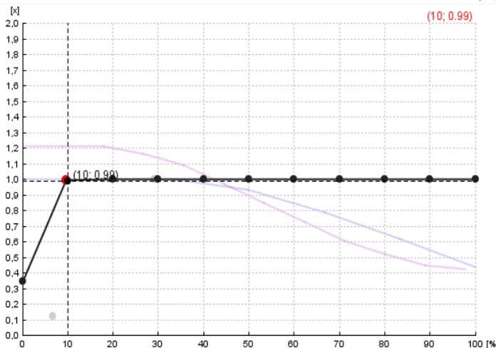
Multiplier Correction (eg. 1.0 is 100%, 0.6 is 60% of original shifting offset) of the angle regarding the TPS signal value.
